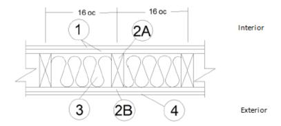
GYPSUM BOARD (Interior): Two layers USG Firecode<sup>®</sup> C Core, complying with ASTM C1396, or equivalent, min. <sup>5</sup>/<sub>8</sub> in. thick, 4ft. wide applied vertically, fastened to framing. Face layer joints staggered with base layer and covered with paper tape and joint compound.
